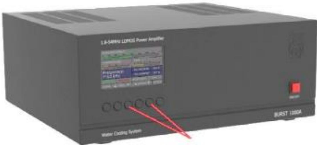
The amplifier BURST 1000A provides 2 types of updates (download link,,,,,,,,,,,,,,,,,,,,,,,,,,,,,,,,,,,,,,,,): graphic/FLASH UPDATE(1) and software/FIRMWARE UPDATE(2), connect Your amplifier to PC via COM Port or USB/COM (you MUST SPECIFY 115200 bps IN the PORT SETTINGS)
